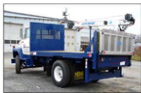
14'6" Body w/ all Electric Crane & 1,600 lbs Rail Lift w/Aluminum Platform
