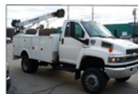
Service Body w/Crane, Liftgate and Pipe Vise
