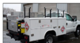
9' Service Body w/ Ladder Rack & 1,500 lbs Aluminum Liftgate
