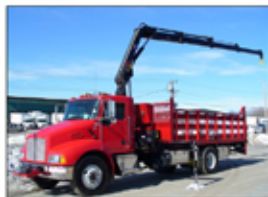
16'6" Body w/ Hiab 111 Crane & 2,000 lbs Rail Lift w/Aluminum Platform
