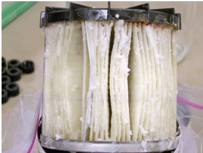
These fuel filters were destroyed by paraffin that precipitated from ultra-low sulfur diesel.
