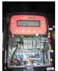
Beckett’s AquaSmart, due out this fall, is meant to conserve energy through the HeatManager system and also make diagnostics easier with its onboard memory and LCD display.
