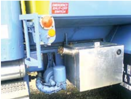
An on-truck injection system is an efficient way to additize fuels.
