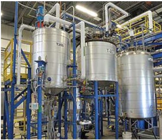
The Biofine process used at the Gorham, Maine, facility results in three useful products: ethyl levulinate which can be used as a fuel; formic acid, which can be sold commercially and a char that can be used to power a facility.
